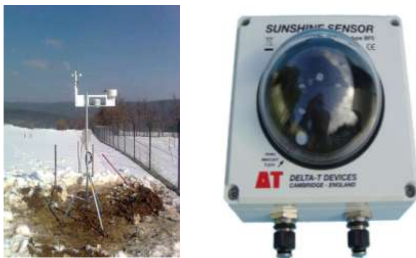
Fig. 1 - Mădârjac Delta-TWeather Station (left) and its radiation sensor (right)
